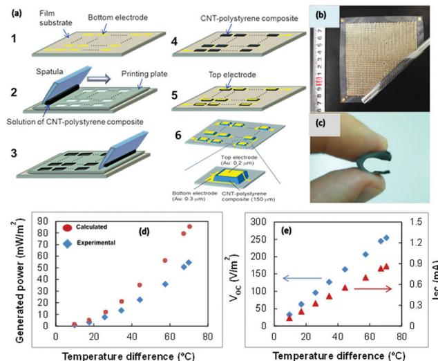
Fig. 9 (a) Schematic of the fabrication steps, (b) photograph of a CNT-polystyrene composite film (thickness:  $75 \mu\text{m}$ ) fabricated on a film substrate, (c) photograph of the fabricated TEG, (d) graph of the generated power output, and (e) open circuit voltage and short-circuit current with temperature difference. Reproduced from ref. 141 (K. Suemori, S. Hoshino, T. Kamata, *Appl. Phys. Lett.* **103** (2013)) with the permission of AIP Publishing.
