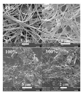
Fig. 4 SEM images of 3 at different water fractions in a  $CH_3CN$ -water mixture (scale bar = 1  $\mu$ m).
