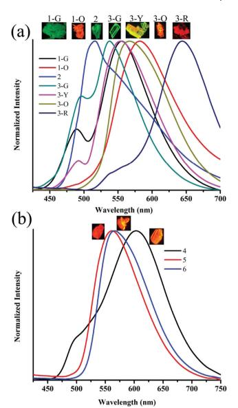
Fig. 5 Solid state fluorescence spectra of (a) **1–3** and (b) **4–6**. Inset shows the digital fluorescence images of crystals.  $\lambda_{\rm exc}$  = 365 nm (for digital images) and 370 nm (for spectra).
