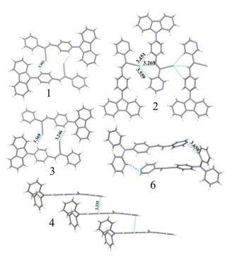
**Fig. 7** Molecular interactions in the crystal lattice of **1–4** and **6**. C (grey), N (blue) and H (white). Dotted lines indicate the hydrogen bonding,  $C-H\cdots\pi$  and  $\pi\cdots\pi$  interactions in Å.
