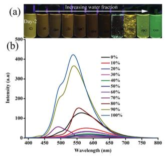
Fig. 2 (a) Digital images and (b) fluorescence spectra of **3** at different water fraction in CH<sub>3</sub>CN:water in day 2.  $\lambda_{\rm exc}$  = 365 nm (for the digital images) and 370 nm (for the spectra).
