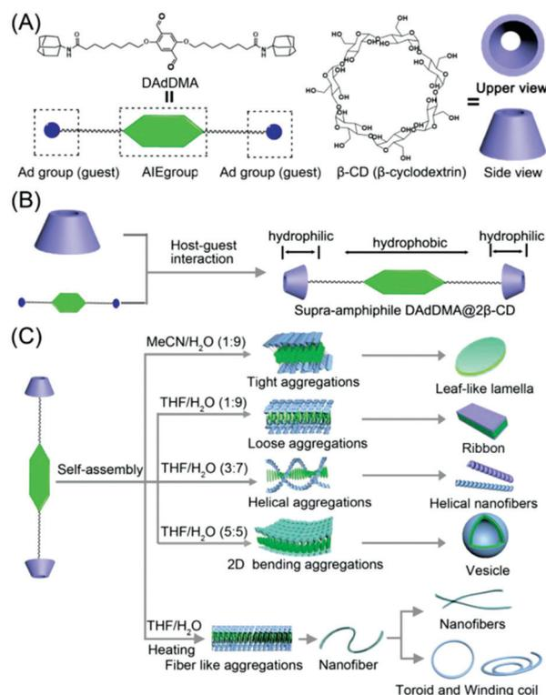
**Scheme 35** (A) The structures of DAdDMA and β-CD. (B) Fabrication of supra-amphiphile DAdDMA@2β-CD. (C) Schematic representation of formation of diversified topological morphologies from DAdDMA@2β-CD supra-amphiphiles. The scheme has been reproduced from ref. 129 with permission from Wiley-VCH Verlag GmbH.
