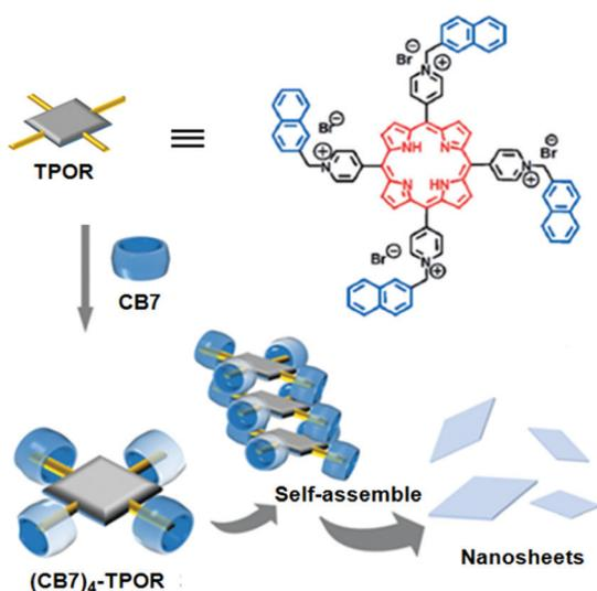
**Scheme 33** Schematic representation of the formation of nanosheets from the interaction of TPOR with CB7. The scheme has been reproduced from ref. 50 with permission from the Royal Society of Chemistry.
