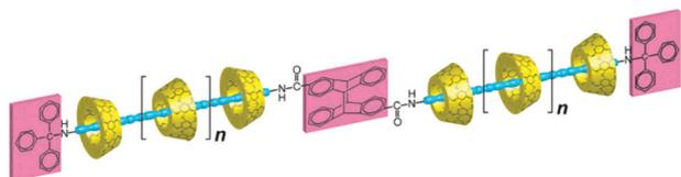
**Scheme 17** Schematic representation of synthesizing  $\alpha$ CD based polyrotaxane *via* photodimerization. The scheme has been reproduced from ref. 97 with permission from the American Chemical Society.
