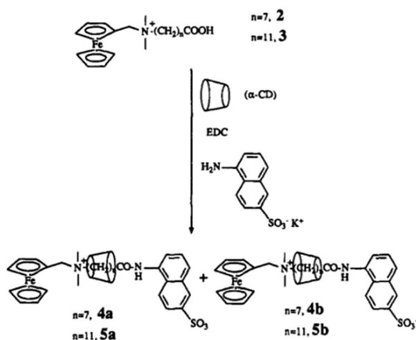
**Scheme 14** Schematic representation of a CD-based rotaxane system, synthesised by capping the free alkanolic acid end by amide coupling. The scheme has been reproduced from ref. 92 with permission from the American Chemical Society.
