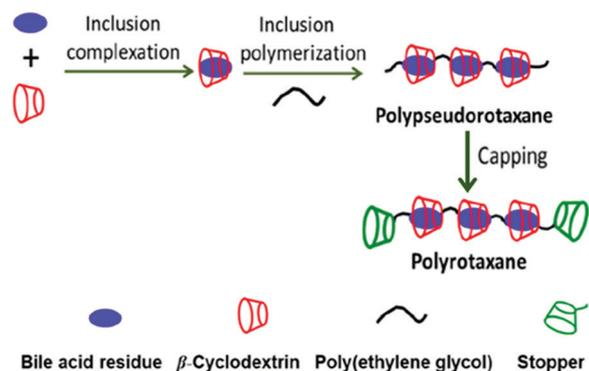
**Scheme 16** Conceptual representation of polyrotaxane formation of  $\beta$ CDs with PEGylated bile acid derivatives. The scheme has been reproduced from ref. 96 with permission from the American Chemical Society.
