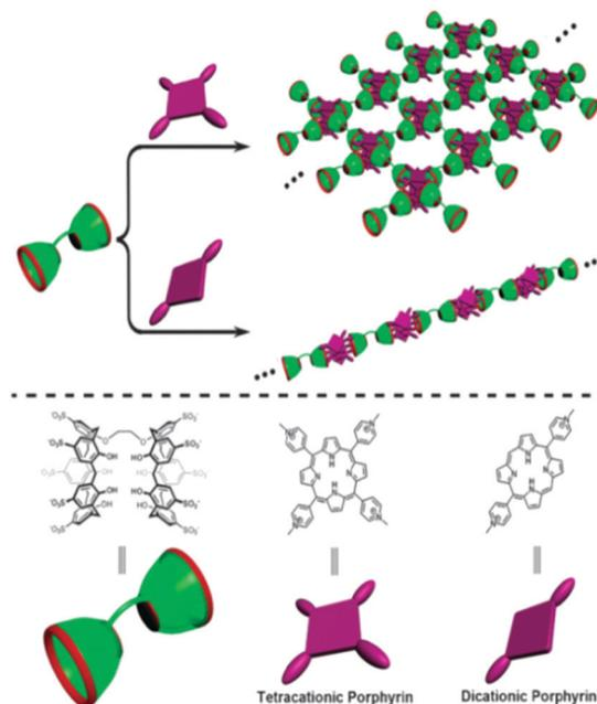
**Scheme 23** Schematic representation of the construction of a supramolecular 2D network and 1D linear polymer based on the complexation of ditopic bis(*p*-sulfonatocalix[5]arene) host with tetracationic and dicationic porphyrin guests, respectively. The scheme has been reproduced from ref. 102 with permission from the Royal Society of Chemistry.
