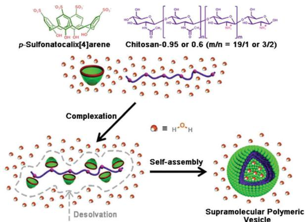
**Scheme 29** Schematic representation of the formation of supramolecular polymeric vesicles by SCX4 and chitosan. The scheme has been reproduced from ref. 121 with permission from Wiley-VCH Verlag GmbH.
