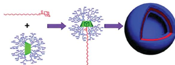
**Scheme 28** Schematic representation of the formation of supramolecular vesicles involving the host-guest interactions of the amphiphilic molecules, CD-*g*-HPG and AD-C18. The scheme has been reproduced from ref. 119 with permission from the American Chemical Society.
