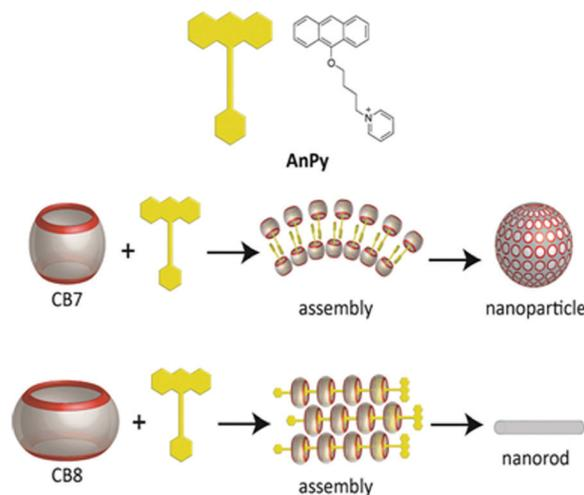
**Scheme 31** Chemical structure of the pyridinium-functionalized anthracene (AnPy) molecule, its symbolic model used and the schematic representation of the supramolecular assemblies formed by the AnPy-CB7 and AnPy-CB8 systems. The scheme has been reproduced from ref. 124 with permission from the Royal Society of Chemistry.
