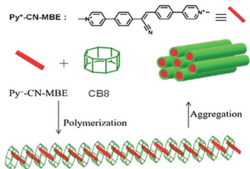
**Scheme 20** Schematic representation of the Py<sup>+</sup>-CN-MBE-CB8 based polymer formation. The scheme has been reproduced from ref. 25 with permission from Wiley-VCH Verlag GmbH.
