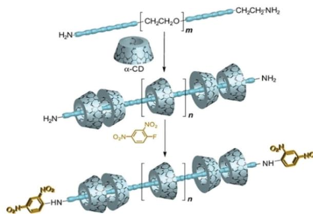
**Scheme 15** Schematic illustration of the synthesis of polyrotaxane incorporating PEG bisamines and  $\alpha$ CD. The scheme has been reproduced from ref. 76 with permission from Wiley-VCH Verlag GmbH.
