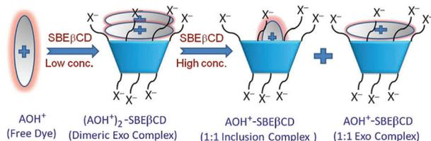
**Scheme 8** Schematic representation of the multistep binding interactions of acridine orange dye ( $\text{AOH}^+$ ) with changing  $\text{SBE}\beta\text{CD}$  host concentration. The scheme has been reproduced from ref. 37 with permission from the Royal Society of Chemistry.
