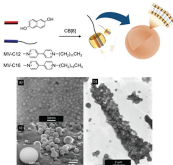
**Scheme 30** Schematic representation of the supramolecular vesicles formed involving ternary complexes of MV-C12 (or MV-C16), DHNp, and CB8. (a) TEM image of the vesicles formed by MV-C12, DHNp, and CB8. (b) TEM and (c) SEM images of the vesicles formed by MV-C16, DHNp, and CB8. The scheme has been reproduced from ref. 122 with permission from Wiley-VCH Verlag GmbH.
