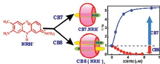
Scheme 5 Schematic representation of the contrasting guest binding interaction of CB7 and CB8 with the NRH<sup>+</sup> dye. The scheme has been reproduced from ref. 63 with permission from the Royal Society of Chemistry.
