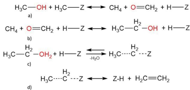
**Scheme 3** Ethene formation *via* methane-formaldehyde mechanism, with (a) methanol and methoxy form methane and formaldehyde, that (b) further convert into ethanol which (c) forms ethoxy and eventually (d) ethene.
