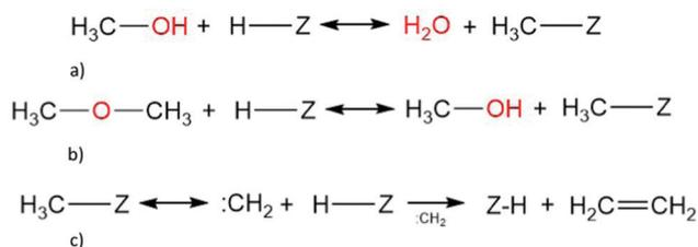
**Scheme 2** Ethene formation *via* methoxy-carbene mechanism, starting from (a) methanol and (b) dimethyl ether to (c) methoxy converted to carbene, finally coupling with another carbene to form ethene.
