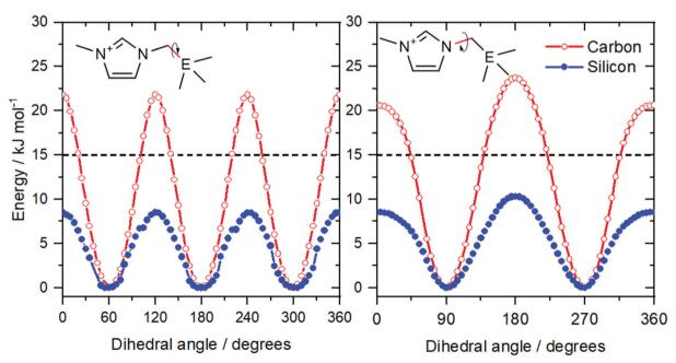
Fig. 8 Energy as a function of the dihedral angles corresponding to rotation around the indicated bonds. Both the N-C and C-E bond rotations benefit from substitution of carbon with silicon; thus reducing the energy barriers by approximately 10 kJ mol<sup>-1</sup>.
