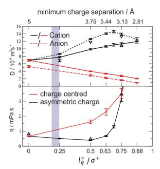
Fig. 16 Diffusion and viscosity as a function of charge separation. The blue shaded area indicates the  $l_a^+/\sigma^+$  range for the [C<sub>4</sub>C<sub>1</sub>im] cation. The charge centred systems where charge separation is achieved by decreasing the size are shown in red. Reprinted (adapted) from H. V. Spohr and G. N. Patey, J. Chem. Phys., 2009, 130, 104506, with the permission of AIP Publishing.217
