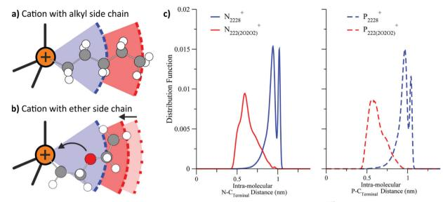
Fig. 9 Cations with alkyl side chains (a) prefer a linear conformation, whereas those with ether side chains (b) coil. (c) For both ammonium and phosphonium ionic liquids, the distance between terminal carbon and quaternary centre is reduced considerably when ether groups are introduced in the side chain. (b) adapted from ref. 140 – Published by the PCCP Owner Societies. (c) Reprinted with permission from ref. 156. Copyright 2013 American Chemical Society.
