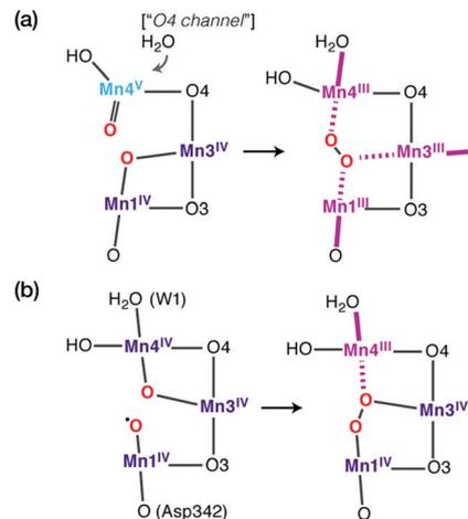
Fig. 9 Schematic depiction of two possibilities for the O–O bond formation step in the  $S_4$  state. (a) Creation of a Mn(V)=oxo species from a preceding water-unbound conformation of the  $S_3$  state enables even-electron intramolecular nucleophilic coupling that resets the cluster to the  $S_0$  oxidation state level. (b) Creation of a Mn(IV)-oxyl intermediate leads to radical oxyl–oxo coupling.
