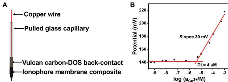
**Fig. 5** Potentiometric characterization of the  $\text{Cu}^{2+}$  ISE: (A) schematic of the carbon-packed  $\text{Cu}(\text{II})$  microsensors. (B) Potentiometric calibration of  $\text{Cu}^{2+}$  with the carbon-packed sensor. DOS: dioctyl sebacate. The sensors showed Nernstian slope of  $29.3 \pm 2.9$  mV/log  $[a_{\text{Cu}^{2+}}]$  and detection limits of  $3.5 \pm 1.0$   $\mu\text{M}$  (number of experiments = 6).
