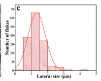
Fig. 1 (a) and (b) SEM images of GNP flakes; (c) Histogram of the lateral flake size for the GNP ink after 70 cycles of microfluidic exfoliation.
