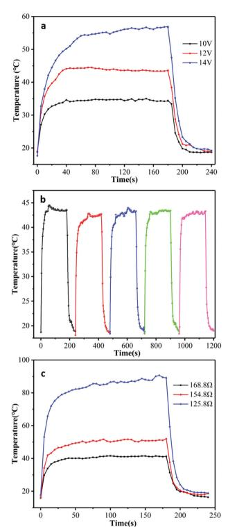
Fig. 4 (a) Temperature profiles of the GNP fabric at different  $V_{\rm GNP}$ ; (b) temperature response of the GNP fabric over 5 cycles at  $V_{\rm GNP}=12$  V, each cycles is 4 min long; (c) temperature profiles of the GNP fabric operated at different biases.
