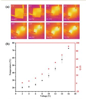
Fig. 3 (a) Infrared thermal images of the conductive fabric at various  $V_{\rm GNP}$ ; (b) plot of the temperature versus  $V_{\rm GNP}$ .
