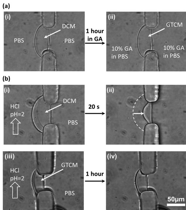
**Fig. 3** GA crosslinking and acidic resistance of DCM and GTCM. (a) No obvious morphological changes were observed after soaking DCM in 10% GA in PBS for one hour to convert it into GTCM. (b)-(i) & (ii) DCM was dissolved by HCl (pH = 2) solution in seconds, while (iii) & (iv) no change in the GTCM was observed under the same condition for one hour.
