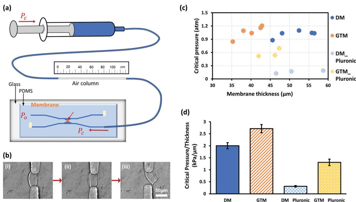
**Fig. 4** Mechanical robustness of DCM and GTCM. (a) Schematic of measurement setup based on Ideal Gas Law to measure the critical pressure to detach membranes from PDMS pillars. (b) Membrane (i) before, (ii) during and (iii) right at the burst moment during a robustness test. (c) Critical pressure of membranes when burst and those after Pluronic treatment. (d) Normalized critical pressure per  $\mu\text{m}$  thickness for different membranes.
