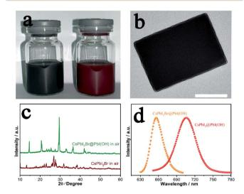
Fig. 4 CsPbl<sub>2</sub>Br prepared by our solution method. (a) Photographs of CsPbl3@Pbl(OH) and CsPbl2Br@Pbl(OH) prepared in solution. (b) TEM image of CsPbl2Br@Pbl(OH). Scale bar: 150 nm. (c) PXRD patterns of CsPbl<sub>2</sub>Br@Pbl(OH) and  $\gamma$ -CsPbl<sub>2</sub>Br in air, showing degradation for the latter, which does not have a PbI(OH) protective shell. (d) Photoluminescence spectra of CsPbI3@PbI(OH) and CsPbI2Br@PbI(OH).
