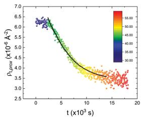
Fig. 5 Time evolution of the  $\rho_{\rm t_{prox}}$  parameter obtained from the analysis of the TTR-NR data measured according to the constant temperature steps profile. Values obtained at different temperatures are labelled with different colors in the graph. The model of the time-dependent kinetic evolution (eqn (5)) is plotted as full line for the temperature range analysed.
