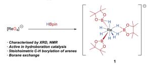
Scheme 1 (A) Selected examples of complexes with boron-centred ligands. (B) This work: synthesis of a rhenium boron-polyhydride anion from HBpin and KReO $_4$ .
