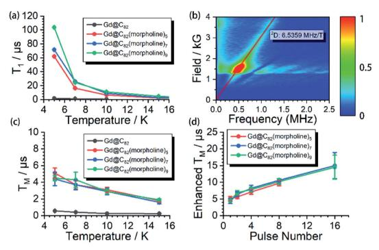
Fig. 3 (a) Spin-lattice relaxation time ( $T_1$ ) of Gd@C<sub>82</sub> and the three derivatives **Gd-n**. (b) 2p-ESEEM spectrum at different external applied magnetic fields for **Gd-5**. The red line represents the simulation with the Lamour frequency of the <sup>2</sup>D nuclear spin. (c) Spin-lattice relaxation time ( $T_1$ ) of Gd@C<sub>82</sub> and the three derivatives **Gd-n**. (d) Dynamic decoupling results for the three derivatives **Gd-n**.
