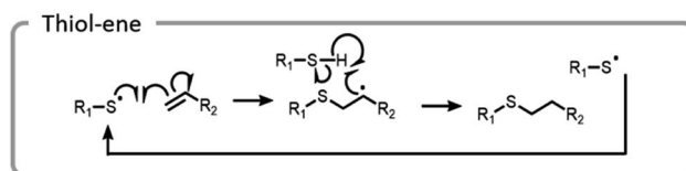
Fig. 12 Mechanism of thiol-ene catalytic reaction.
