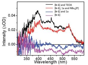
Fig. 2 Transient absorption studies on PCET-mediated N-radical generation at 10  $\mu$ s time delay.
