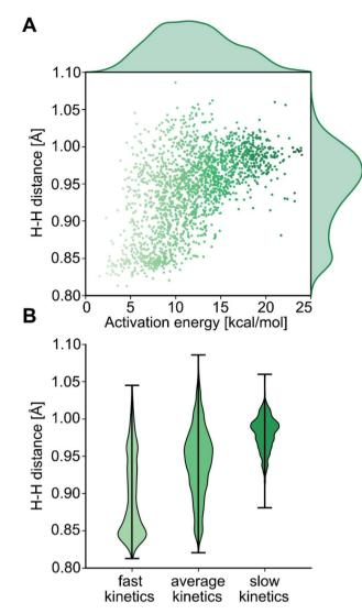
Fig. 4 (A) Correlation and distributions of energy barriers and H–H distances at the transition state. (B) Distributions of H–H distances for the arbitrary kinetics categories 'fast' ( $\Delta E_{\rm HH}^{\dagger} < 8.1$  kcal mol<sup>-1</sup>), 'average' (8.1 kcal mol<sup>-1</sup> <  $\Delta E_{\rm HH}^{\ddagger} < 15.1$  kcal mol<sup>-1</sup>) and 'slow' ( $\Delta E_{\rm HH}^{\ddagger} > 15.1$  kcal mol<sup>-1</sup>).
