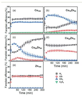
Fig. 2 Time-dependencies of the Faradaic efficiency of the main reaction products for  $CO_2RR$  at -1.35 V vs. RHE for Cu NPs (a),  $Cu_{70}Zn_{30}$  NPs (b),  $Cu_{50}Zn_{50}$  NPs (c),  $Cu_{30}Zn_{70}$  NPs (d) and Zn NPs (e).
