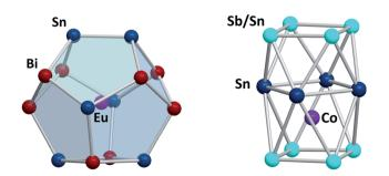
Fig. 7 From left: molecular structures of the cluster anions [Eu@Sn<sub>6</sub>Bi<sub>8</sub>] $^{4-}$ ,136 and [Co@Sn<sub>6</sub>Sb<sub>6</sub>] $^{4-}$ .141 The clusters show positional disorder of the main group elements in the cluster shell. The atom distributions depicted here are based on quantum chemical calculations and represent the energetically preferred distribution.
