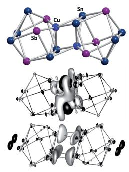
**Fig. 8** Top: molecular structure of the cluster anion  $[(CuSn_5Sb_3)_2]^{4-}$ . Late Center and bottom: difference of electron densities of dimer and monomers upon hypothetic dimerization reactions to form  $[(CuSn_5Sb_3)_2]^{4-}$  or the non-existent " $(Sn_9^{2-})_2$ " analogue. Contours are drawn at 0.0016 a.u. For black areas, electron density in the dimer is higher than in the monomers, for light areas it is lower (reproduced from ref. 142 with permission from Wiley-VCH).
