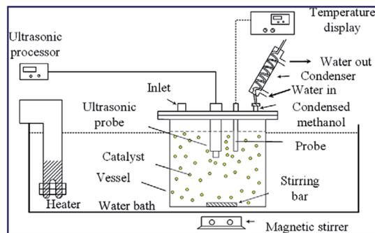
Fig. 3 Schematic portrayal of experimental set up for the ultrasonic-assisted transesterification reaction. Reproduced from ref. 86.
