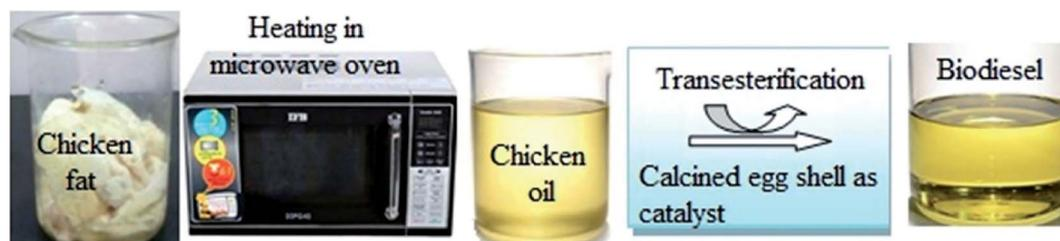
Fig. 14 Microwave-assisted synthesis of FAME using an eggshell catalyst. Reproduced from ref. 190.
