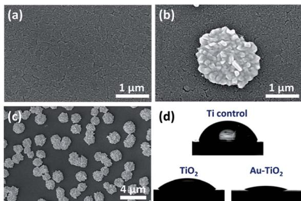
Fig. 2 SEM image of (a) TiO<sub>2</sub> and flower-like hierarchical Au structures modified TiO<sub>2</sub> at (b) high and (c) low magnification. (d) Images for contact angle properties of prepared samples.
