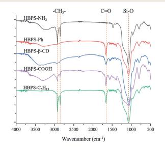
Fig. 1 FT-IR spectral characterization of HBPS-NH<sub>2</sub>, HBPS-Ph, HBPS- $\beta$ -CD, HBPS-C<sub>6</sub>H<sub>13</sub> and HBPS-COOH.
