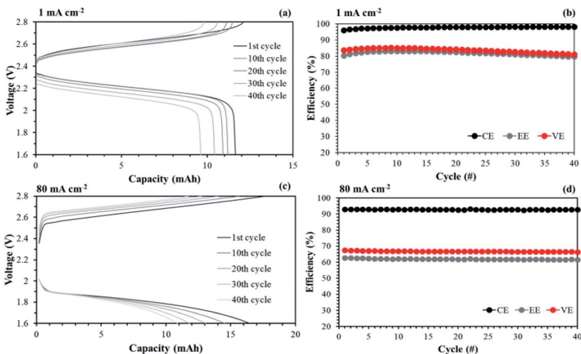
Fig. 16 Comparison of performances in a single cell using 0.05 M  $V(acac)_3/TEABF_4$  at  $60 \text{ mL min}^{-1}$ : (a) charge/discharge curves and (b) efficiencies by applying AHA membrane; (c) charge/discharge curves and (d) efficiencies by introducing the aligned cQPPO membrane at 1.5 V.
