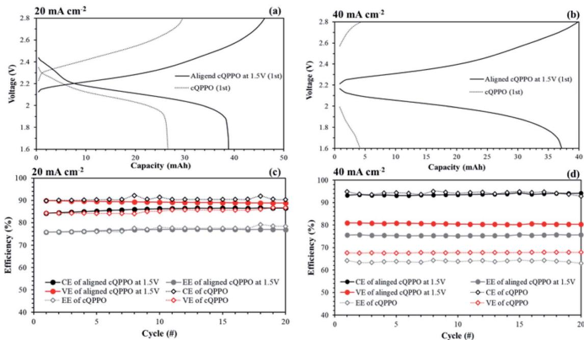
Fig. 15 Comparison of performances in a single cell using 0.05 M  $V(acac)_3/TEABF_4$  at  $60 \text{ mL min}^{-1}$ : (a) charge/discharge curves at (a) 20 and (b) 40  $\text{mA cm}^{-2}$ ; efficiencies at (c) 20 and (d) 40  $\text{mA cm}^{-2}$  by applying the non-aligned and aligned cQPPO membrane.
