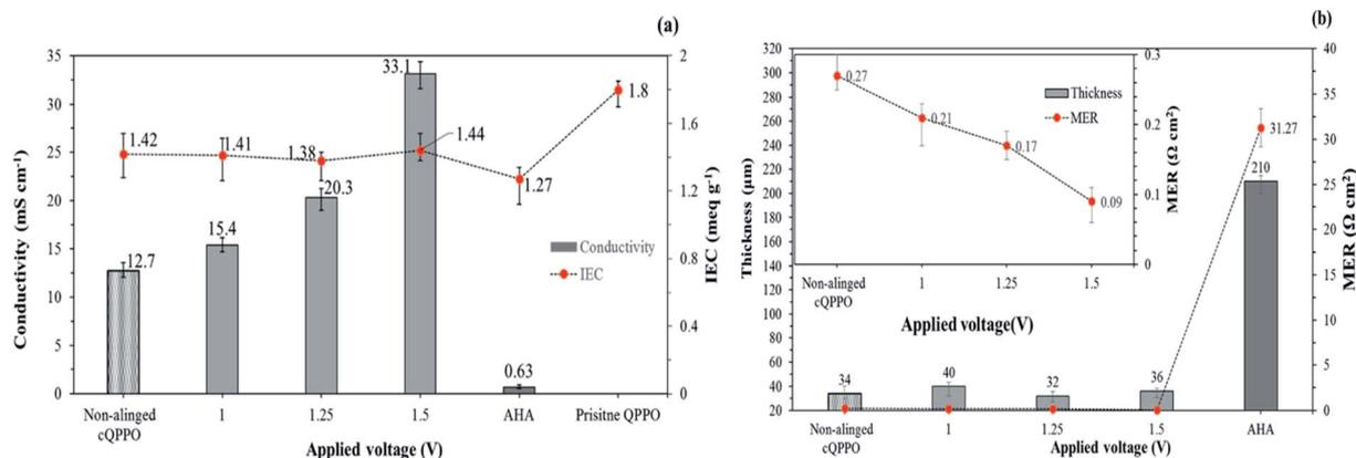
Fig. 8 (a) Ion exchange capacity and through-plane conductivity for fabricated membranes according to the intensity of the electrical treatment and AHA in 1 M TEABF<sub>4</sub> in ACN; (b) comparison of the MER of fabricated membranes and commercial AHA membrane.
