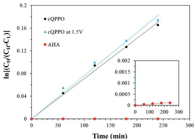
Fig. 19 Comparison of the concentration changes in  $\text{V}(\text{acac})_3$  on the deficient side with the elapsed time for the three types of membranes.
