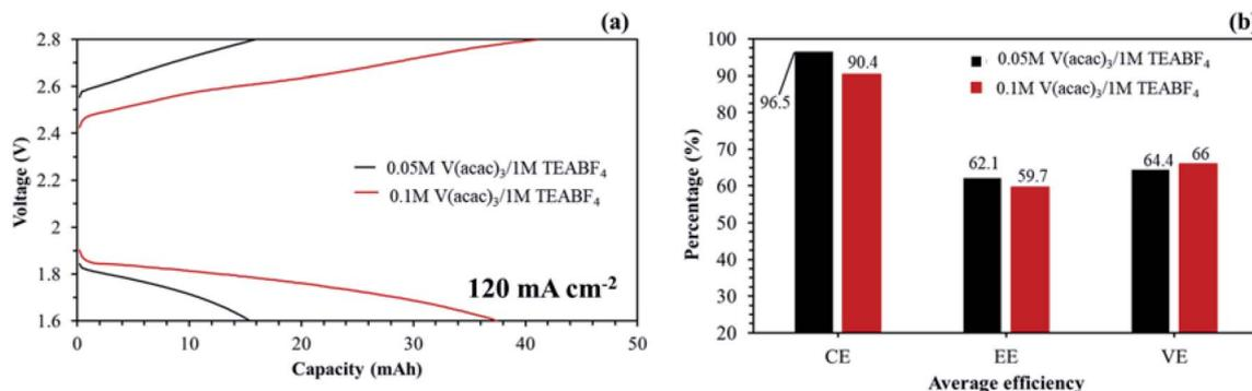
Fig. 18 Single cell performances on the application of the aligned cQPPO at  $120 \text{ mA cm}^{-2}$  with  $120 \text{ mL min}^{-1}$ : (a) capacity–voltage curves of the NAVRFB assembled with the aligned cQPPO membrane; (b) average efficiencies in 40 cycles.
