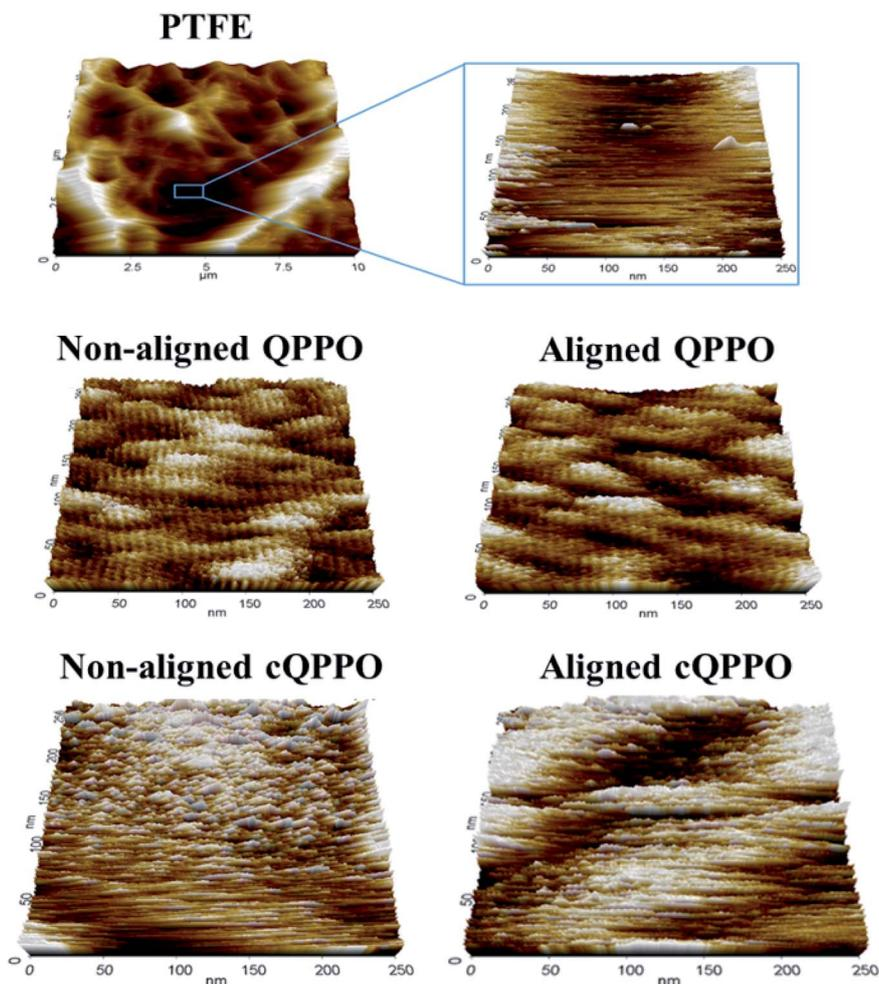
Fig. 13 Morphological AFM image of fabricated membranes: (a) the porous PTFE; (b) empty space of porous substrate; (c) casting QPPO; (d) aligned QPPO at  $31 \text{ V cm}^{-1}$ ; (e) non-aligned and (f) Aligned cQPPO at  $1.5 \text{ V}$  (about  $31 \text{ V cm}^{-1}$ ).
