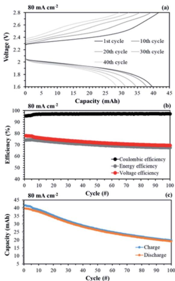
Fig. 17 Performances of a single cell with  $0.05\ \text{M V}(\text{acac})_3/1\ \text{M TEABF}_4$  at a high flow rate ( $120\ \text{mL min}^{-1}$ ): (a) capacity–voltage curves; (b) efficiencies and (d) capacity changes of long-term operation, by applying the aligned cQPPO at  $1.5\ \text{V}$ .
