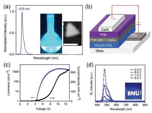
Fig. 13 (a) PL spectrum of the CDs. Insets: Photographs under UV light (left) and HAADF-STEM image of the CDs. (b) Device structure of the CD-LEDs. (c) L-J-Vcharacteristic of the CD-LEDs. (d) EL spectra of the blue-LEDs at different bias voltages. Reproduced with permission. <sup>123</sup> Copyright 2018, Nature Publishing Group.
