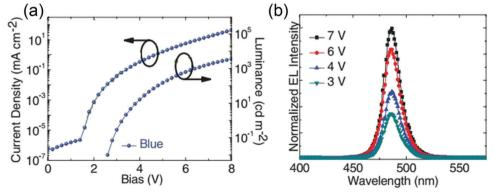
Fig. 8 (a) J-L-V characteristics for blue PeLEDs based on Cs-doped MA<sub>0.17</sub>FA<sub>0.83</sub>Pb(Br<sub>x</sub>l<sub>1-x</sub>)<sub>3</sub>. (b) EL spectra of the blue-colored PLEDs operating at various voltages. Reproduced with permission. 66 Copyright 2017, John Wiley & Sons, Inc.
