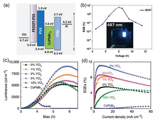
Fig. 9 (a) Energy diagrams for ITO/PEDOT: PSS/PVK/BA<sub>2</sub>Cs<sub>n-1</sub>Pb<sub>n</sub>(Br/X)<sub>3n+1</sub>/TPBi/Al LEDs. (b)  $\eta_{EQE}$ -voltage for B487 LEDs for champion devices. Inset: Photos of these LEDs. Reproduced with permission. curves of CsPbBr<sub>3</sub>: PEACl (1:1) devices with different ratios of YCl<sub>3</sub>. Reproduced with permission. <sup>81</sup> Copyright 2019, Nature Publishing Group.
