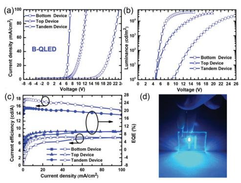
Fig. 6 (a) J-V characteristics, (b) L-V characteristics, and (c) current efficiency  $-J-\eta_{\text{EQE}}$  characteristics of the blue QD-LEDs. (d) Photos of the tandem blue QD-LEDs operated at a current density of 100 mA cm<sup>-2</sup>. Reproduced with permission.<sup>54</sup> Copyright 2017, American Chemical Society.
