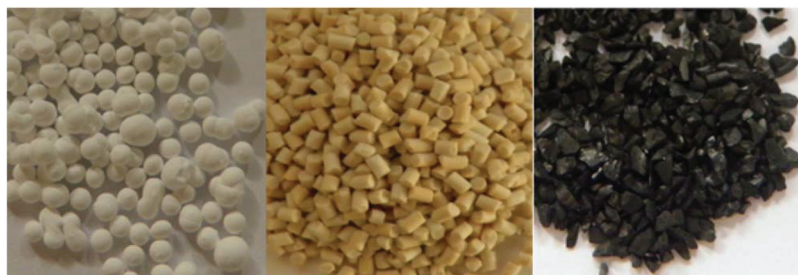
Fig. 4 The photographs of UiO-66-COOH beads obtained by freeze granulation (left) and extrudates (center), and of commercial type K adsorbent (activated carbon) from 3 M (right). Reprinted with permission from ref. 106. Copyright 2018 American Chemical Society.
