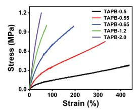
Fig. 3 Typical stress-strain curves of TAPB.
