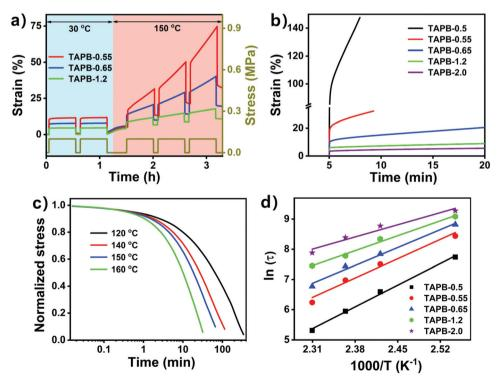
Fig. 4 (a) Cyclic strain/recovery profiles of TAPB-0.55, TAPB-0.65 and TAPB-1.2 at 30 and 150 °C with a stress of 0.1 MPa. (b) Creep experiments for TAPB with a constant stress of 0.15 MPa at 150 °C. (c) Stress relaxation curves for TAPB-0.65 at different temperatures under a constant strain of 2%. (d) Fitting of  $\tau$  to the Arrhenius law for TAPB.
