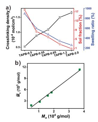
Fig. 2 (a) Crosslinking density, sol fraction and swelling ratio of TAPB. (b) Relationship between  $\bar{M}_c$  of TAPB and  $M_n$  (determined by <sup>1</sup>H NMR) of APB.
