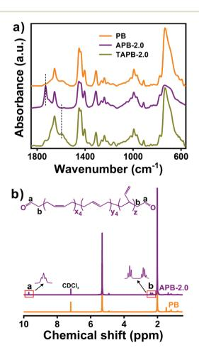
Fig. 1 (a) FTIR spectra of PB, APB-2.0 and TAPB-2.0. (b)  $^1\mathrm{H}$  NMR spectra of PB and APB-2.0.
