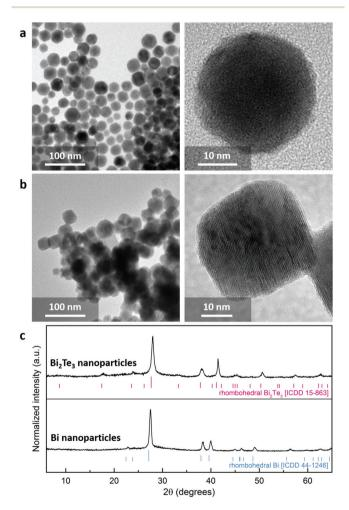
Fig. 2  $Bi_2Te_3$  nanoparticle synthesis: (a) TEM images of Bi nanoparticles, which are nearly spherical and of average radius 14.4 nm. (b) Successfully synthesized  $Bi_2Te_3$  nanoparticles with a slightly rhombohedral shape and average radius of 17.5 nm. (c) X-ray diffraction patterns illustrating the successful tellurisation of the Bi nanoparticles to form  $Bi_2Te_3$  nanoparticles.
