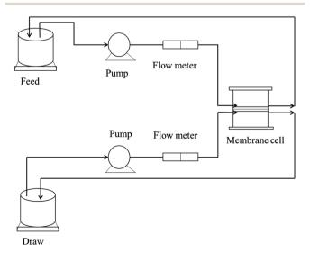
Fig. 3 Schematic diagram of the FO lab-scale system.<sup>26</sup>
