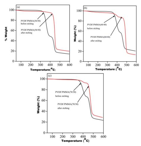
Fig. 4 TGA profiles of blends before and after etching of PMMA from PVDF/PMMA blends with different compositions: (a) 50/50, (b) 60/40 and (c) 70/30.
