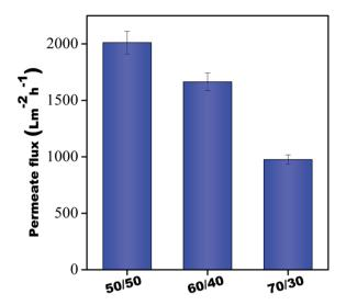
Fig. 7 Pure water flux of all individual membranes
