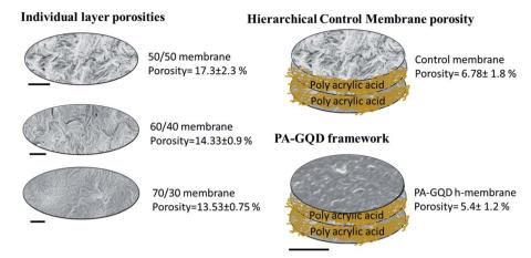
Fig. 15 Role of individual layers and their arrangement in selectively remediating dye pollutants and salt ions. The scale bar indicated is 2 µm.
