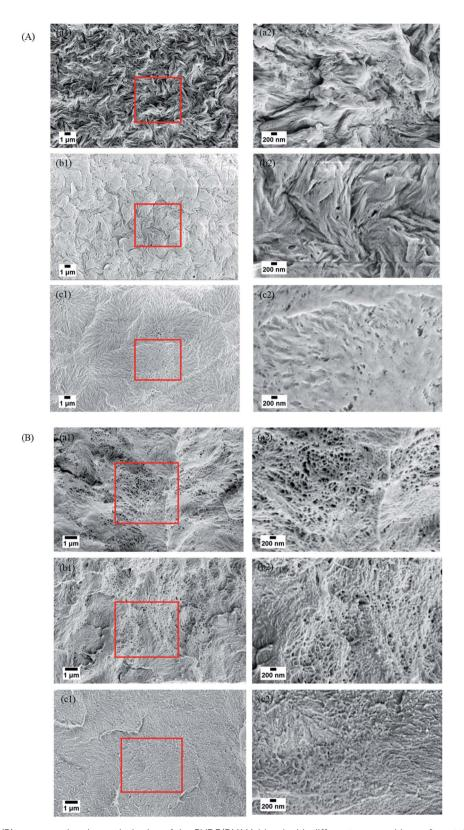
Fig. 5 (A) Surface and (B) cross-sectional morphologies of the PVDF/PMMA blend with different compositions after etching with glacial acetic acid for 7 days. (a) 50/50, (b) 60/40 and (c) 70/30.
