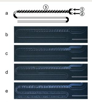
Fig. 1 Temperature-dependent mixing of 5CB and MeOH, infused at the top (a1) and bottom (a2) inlet, respectively. Passive mixing was induced via a static micromixer with staggered oriented ridges (a3). (be) Snapshots of the microfluidic chip at various temperatures: 40 °C (b); 35 °C (c); 24 °C (d) and 12 °C (e).
