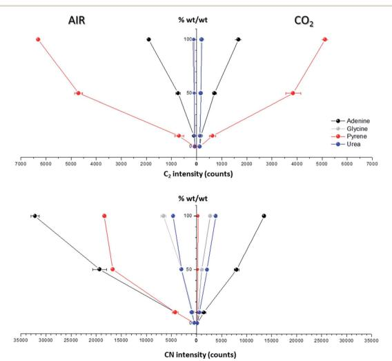
Fig. 2 Effect of the concentration of C-containing dopants (adenine, glycine, pyrene and urea) on optical emission of molecular bands ( $C_2$  473.70 mm and CN 388.30 nm). Measurements were conducted under two different atmospheric conditions: in air and in CO<sub>2</sub>, both at 7 mb. The laser fluence was fixed at 72.4 J cm<sup>-2</sup>.
