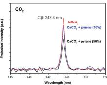
Fig. 4 Emission intensity of the atomic carbon signal from both the pure CaCO<sub>3</sub> matrix and that doped with 10% pyrene in both air and the CO<sub>2</sub> atmosphere.
