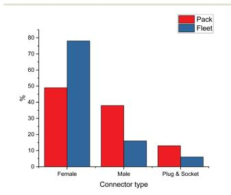
Fig. 9 (red) Proportion of packs utilising each intermodular connection type, (blue) proportion of connection type across fleet population of modules. Data from 2018 EU sales of (H)EVs where available.
