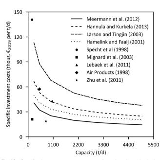
Fig. 10 Specific investment cost curves of methanol synthesis loop including purification normalized to the year 2019. 228,232,239-245
