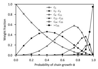
Fig. 20 Anderson-Schulz-Flory distribution: weight fraction of different carbon number products as a function of the chain growth  $\alpha$ .  $\alpha$  is among other things influenced by the catalyst, the reaction conditions, the temperature and the syngas stoichiometry. Adapted from ref. 351-353.
