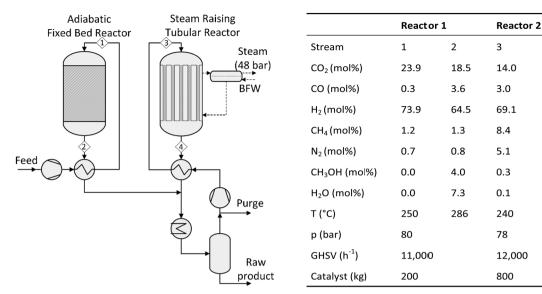
Fig. 9 Simplified scheme and process parameters of the Lurgi two-stage process for methanol synthesis from  $CO_2$  (own illustration based on König and Göhna<sup>194</sup>).
