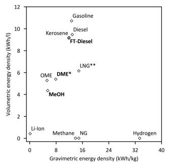
Fig. 1 Gravimetric and volumetric energy density of different fuels and Li-Ion batteries for comparison (\*at 10 bar; \*\*at -160 °C).  $^{13-15}$
