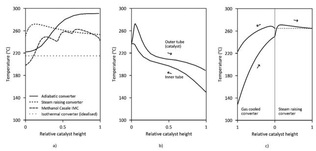
Fig. 7 Temperature profiles along the reactor length of (a) adiabatic converter, 105 steam raising converter, Methanol Casale IMC, 142 and isothermal converter (idealized), (b) Mitsubishi Superconverter, 143 (c) Lurgi MegaMethanol. 99
