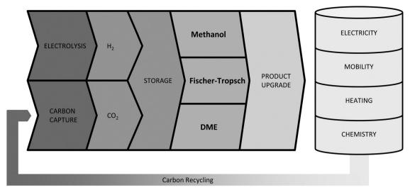
Fig. 2 Power-to-X pathways to transform electricity to chemicals via electrolysis and synthesis. The power-to-X principle connects different energy sectors via carbon capture from industrial plants or chemical/natural (photosynthesis)  $CO_2$  scrubbing from the air, the carbon cycle can be closed so that no additional  $CO_2$  is emitted. This paper regards paths to transform electricity to liquid fuels for the mobility sector.
