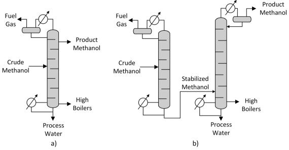
Single column (a) and two-column (b) methanol distillation, own illustration based on Supp. 55
