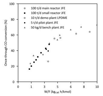
Fig. 17 Dependency of once-through CO conversion on catalyst loading ratio W/F (catalyst weight/reactor inlet gas flow rate) of JFE plants (260  $^{\circ}$ C, 50 bar)<sup>258</sup> and LPDME 10 t per d demonstration (own calculation based on ref. 261).
