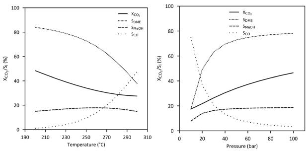
Fig. 13 Equilibrium conversion of CO<sub>2</sub> (=  $[CO_{2,in} - CO_{2,out}]/CO_{2,in}$ ) and selectivity of DME, methanol and CO ( $S_i = i/[CO_{2,in} - CO_{2,out}]$ , with i = 12 × DME/MeOH/CO, based on amount of C-atoms) dependent on (a) temperature and (b) pressure (H<sub>2</sub>: CO<sub>2</sub> = 3:1, based on Aspen Plus Simulation).
