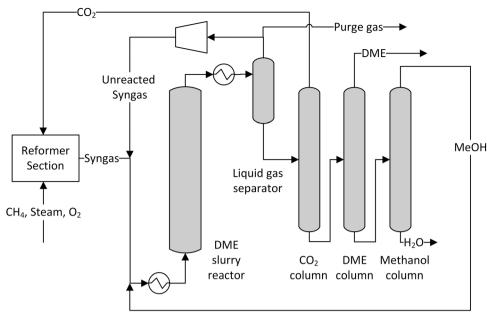
Fig. 16 Schematic process flow of the JFE 100 t per d demonstration plant (own illustration based on Yagi et al. <sup>258</sup>).
