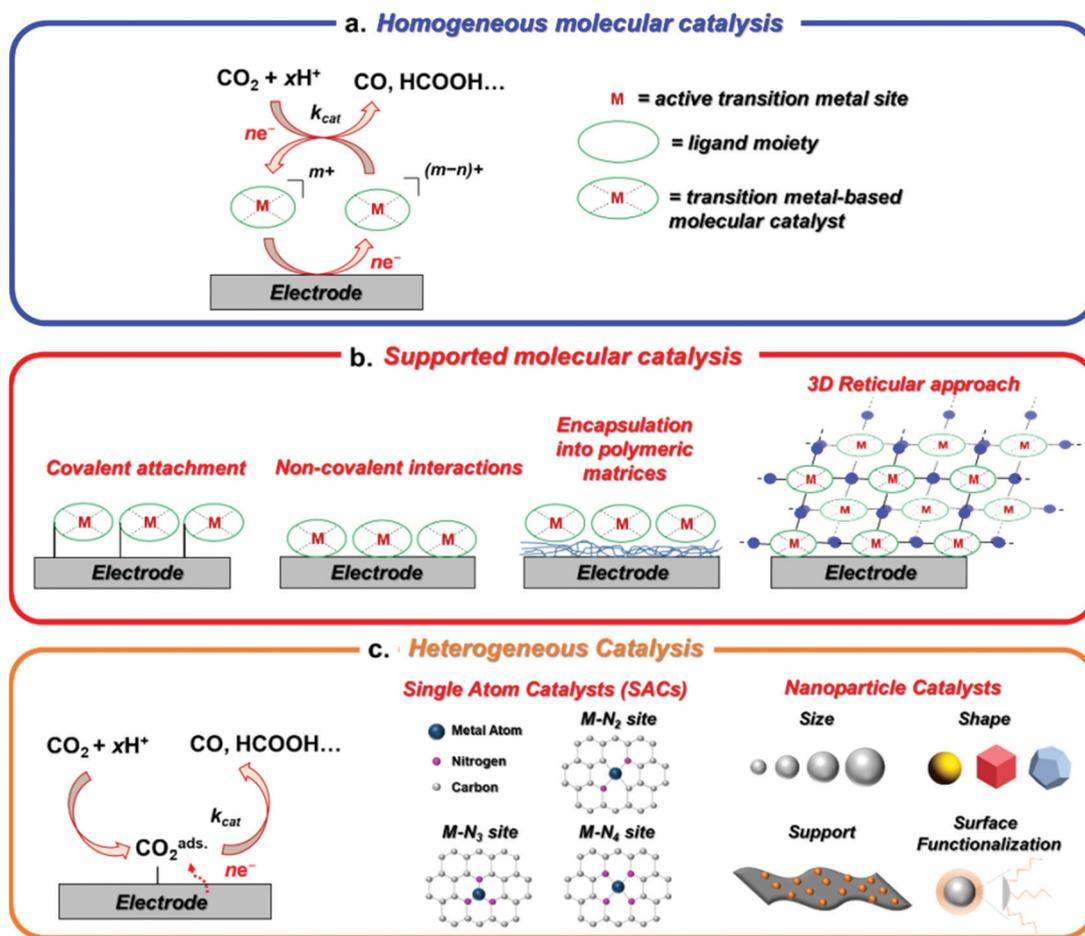
Fig. 1 Different types of transition metal catalysts for CO<sub>2</sub>RR: (a) homogeneous molecular catalysis, (b) surface-anchored molecular catalysis by using several immobilization strategies and (c) heterogeneous catalysis.
