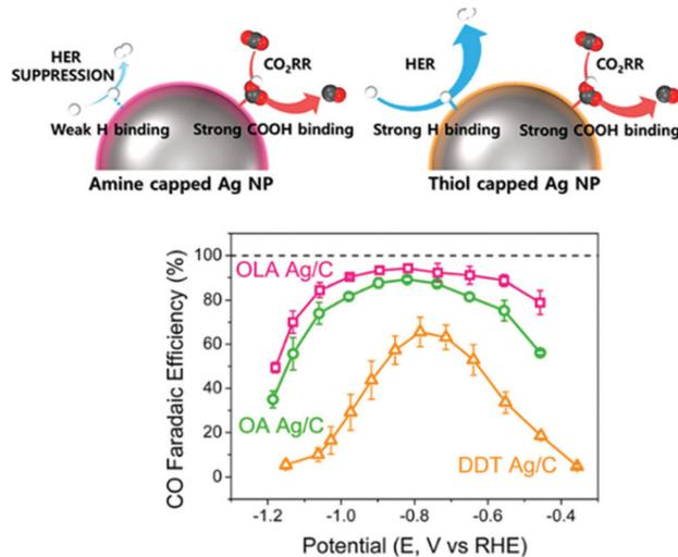
Fig. 33 Schematic illustration of amine- and thiol-capped Ag NPs for  $\text{CO}_2\text{RR}$ . CO faradaic efficiency as a function of the applied potential for oleylamine (OLA)-capped Ag/C, oleic acid (OA)-capped Ag/C, and dodecanethiol (DDT)-capped Ag/C. Reproduced with permission from ref. 424. Copyright 2017 American Chemical Society.
