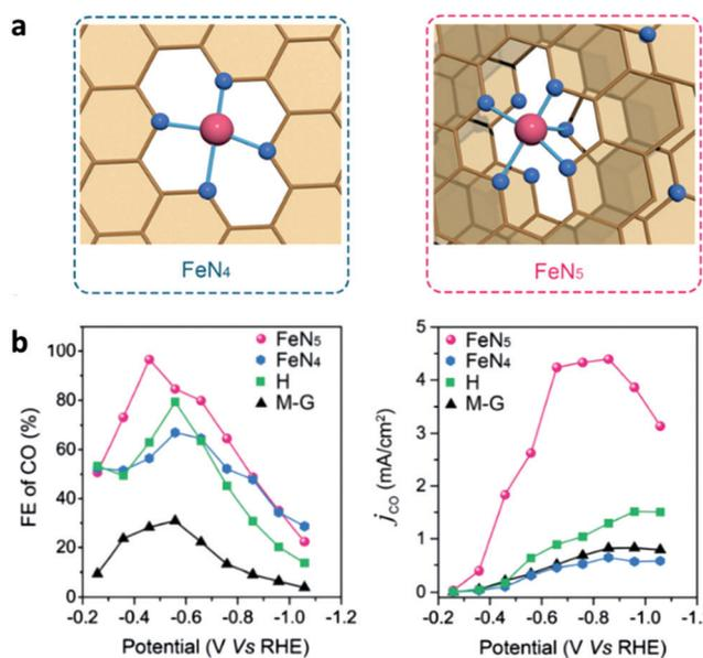
Fig. 24 (a) Scheme of the FeN<sub>4</sub> and FeN<sub>5</sub> catalysts. CO<sub>2</sub>RR catalytic performance of the as-synthesized catalysts. (b) Faradaic efficiency and partial current density for FeN<sub>5</sub>, FeN<sub>4</sub>, and the precursors hemin (H) and melamine with graphene (M–G). Adapted with permission from ref. 344. Copyright 2019, Wiley–VCH.
