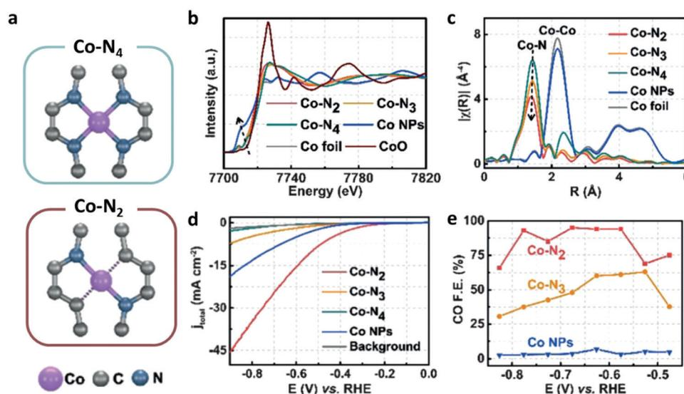
Fig. 26 (a) Schemes of Co–N<sub>4</sub> and Co–N<sub>2</sub>. (b) XANES (c) EXAFS spectra suggesting the atomic dispersion of Co atoms in Co–N<sub>2</sub>, Co–N<sub>3</sub>, and Co–N<sub>4</sub>, and the lowest N coordination number in Co–N<sub>2</sub>. (d) LSV of Co–N<sub>2</sub>, Co–N<sub>3</sub>, Co–N<sub>4</sub>, and Co NPs and pure carbon paper as background. (e) CO faradaic efficiencies at different applied potentials. Adapted with permission from ref. 359. Copyright 2018, Wiley-VCH.
