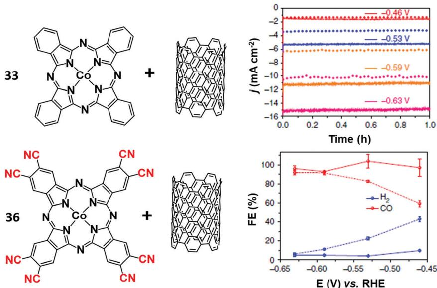
Fig. 10 Comparison of the CO<sub>2</sub>RR performances of CoPc (**33**) and the CN-functionalized derivative **36** anchored to a MWCNT electrode in aqueous electrolyte (0.1 M KHCO<sub>3</sub>). Chronoamperograms (top right) and FEs (bottom right) of CO<sub>2</sub>RR products at different potentials for CoPc-CN/CNT (solid line) in comparison with CoPc/CNT (dotted line). Adapted with permission from ref. 184. Copyright 2017, Nature Publishing Group.
