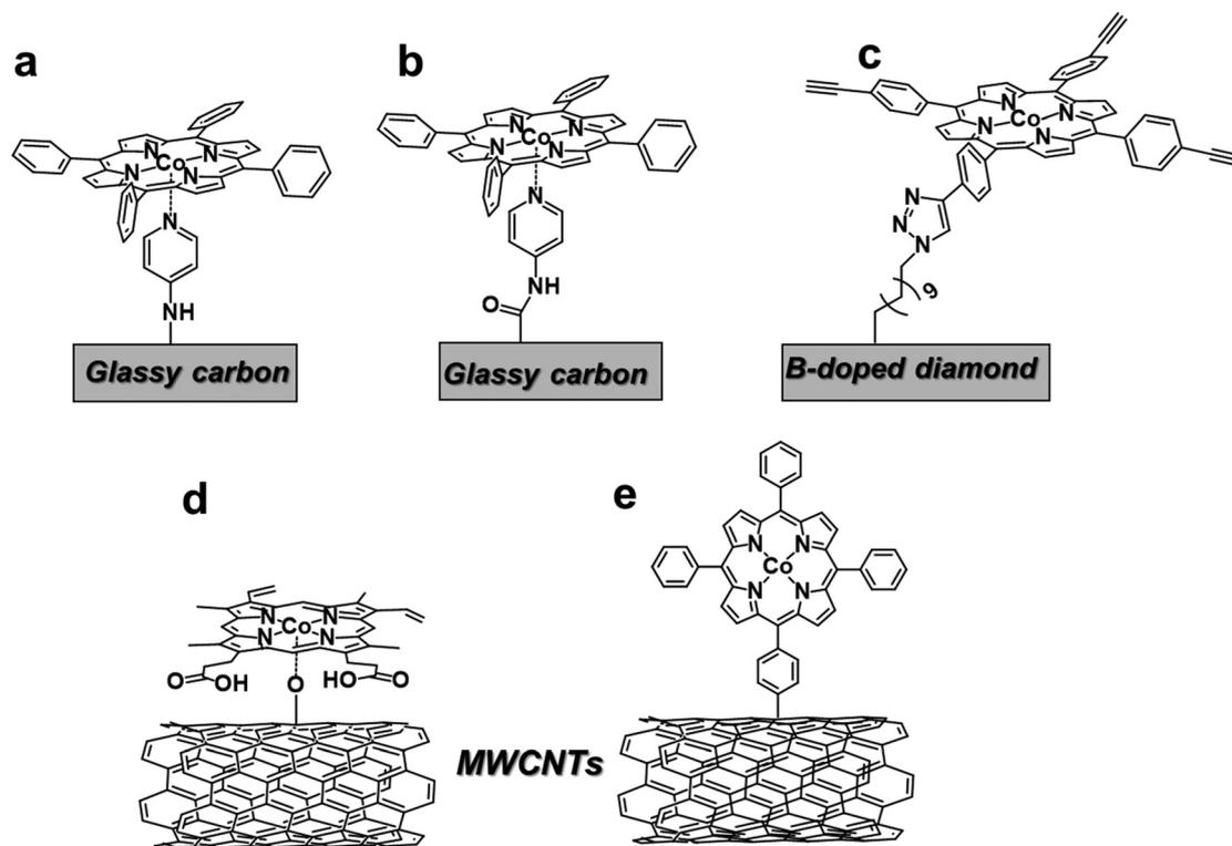
Fig. 7 Different proposed strategies for covalent attachment of Co porphyrin catalysts for  $\text{CO}_2\text{RR}$ . Pictorial representation of catalysts reported in ref. 73 and 159–162.
