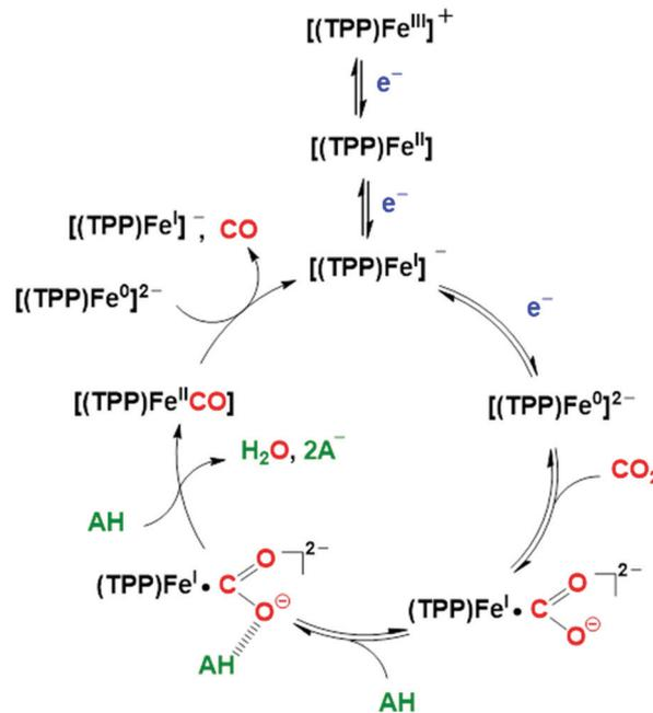
Scheme 1 Proposed catalytic mechanism for the electrochemical CO<sub>2</sub>-to-CO mediated by [Fe(TPP)Cl] (**1**) in organic media in the presence of Brønsted acids.<sup>86,102</sup>
