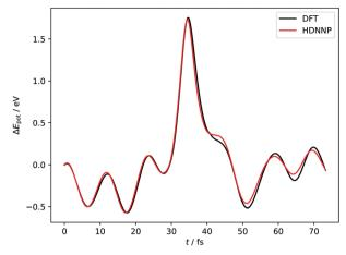
Fig. 4 Potential energies from AIMD and HDNN-PES trajectories with  $E_i = 1.9 \text{ eV}$ ,  $\theta_i = 34^\circ$  and  $\phi_i = 0^\circ$ . The two trajectories were launched with identical initial conditions and both traverse the chemisorption well before returning to the gas phase after a single bounce. The distance of closest approach is below  $r_{CH} = 1.4 \text{ Å}$ . Movies of the two trajectories can be found in the ESI.†
