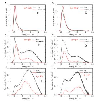
Fig. 8 Comparing theory with experiment: angle integrated energy loss spectra. All incidence conditions are the same as in Fig. 6.
