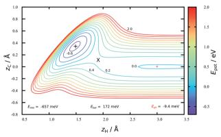
Fig. 2 A cut through the HDNN-PES in the vicinity of the minimum energy path to chemisorption. The H atom is constrained to lie directly above a C-atom.  $z_H$  and  $z_C$  indicate the distance of H and C, respectively, from the plane of the graphene sheet. The physisorption (+) and chemisorption (+) minima have depths of 9 and 657 meV, respectively. The barrier to chemisorption (x) has a height of 172 meV.
