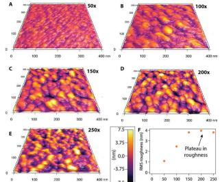
Fig. 2 AFM images of lithicone films at (a) 50, (b) 100, (c) 150, (d) 200, (e) 250 deposition cycles. (f) RMS roughness as a function of MLD cycle number is shown.
