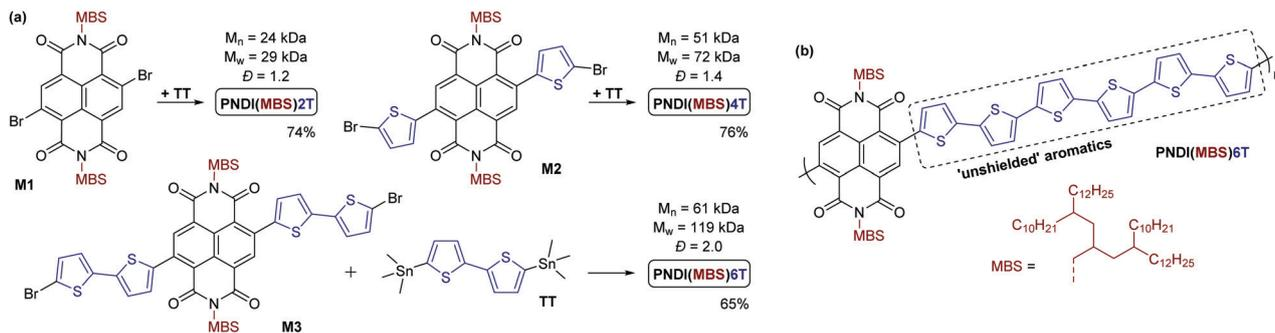
**Scheme 3** (a) Stille copolymerization of monomers **M1**, **M2**, and **M3** with distannylated bithiophene **TT** yielding polymers **PNDI(MBS)2T**, **PNDI(MBS)4T**, and **PNDI(MBS)6T**, respectively. Polymerization conditions: Pd<sub>2</sub>(dba)<sub>3</sub>, P(*o*-tol)<sub>3</sub>, chlorobenzene, 100 °C → 200 °C, microwave oven. (b) Structure of **PNDI(MBS)6T** with highlighted unsubstituted, 'unshielded' thiophene units.
