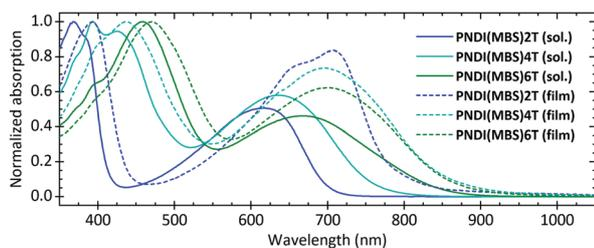
**Fig. 1** Normalized UV-vis absorption spectra of **PNDI(MBS)2T-6T** in CB (0.1 g L<sup>-1</sup>) and as annealed films.
