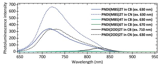
**Fig. 2** Photoluminescence spectra of **PNDI(MBS)2T-6T** and **PNDI(2OD)2T** in chlorobenzene (CB) and chloronaphthalene (CN). Conc.: 0.1 g L<sup>-1</sup>.
