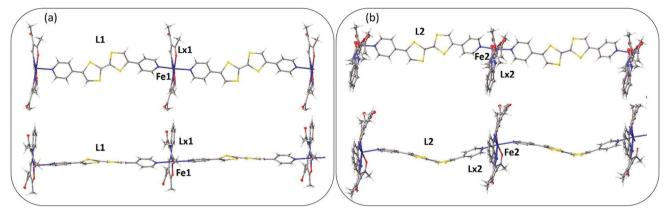
Fig. 2 Structural representation (100 K) of the coordination polymer chains of [FeLa(py2TTF)]<sub>n</sub> formed by (a) Fe1-L1-La1 and (b) Fe2-L2-La2, highlighting the linear versus undulating chain motifs directed by the difference in L1 and L2 geometries. Each chain is shown in two different orientations.
