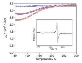
Fig. 5  $\chi_{\rm M}T$  vs. T plot of [FeL<sub>a</sub>(py<sub>2</sub>TTF)]<sub>n</sub> (red) and doped with iodine for 2 days (purple) and 2 weeks (blue). Inset: EPR spectrum of [FeLa(py2TTF)]<sub>n</sub> infused with iodine for 2 weeks showing an oxidised TTF signal.
