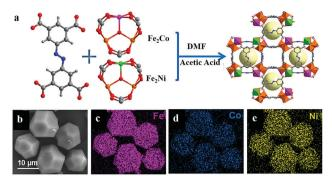
Fig. 1 (a) Schematic diagram of the synthesis of PCN-Fe<sub>2</sub>Co-Fe<sub>2</sub>Ni. (b) Scanning electron microscopy (SEM) image and (c-e) corresponding elemental (Fe, Co and Ni) mapping images for PCN-Fe<sub>2</sub>Co-Fe<sub>2</sub>Ni. Adapted with permission from (ref. 82). Copyright (2019) American Chemical Society
