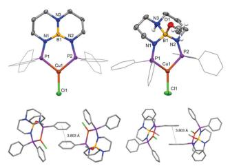
Fig. 1 Top: Molecular structures of 1 (left) and 1-MeOH (right) with thermal ellipsoids at the 50% probability level. Phenyl groups are depicted as wire frames, and hydrogen atoms except for NH and OCH<sub>3</sub> were omitted from the figures. Bottom: Intermolecular  $\pi$ - $\pi$  stacking in the extended XRD structure of 1-MeOH.
