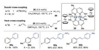
Scheme 22 Dinuclear Pd-catalyzed Suzuki and Heck cross-coupling
