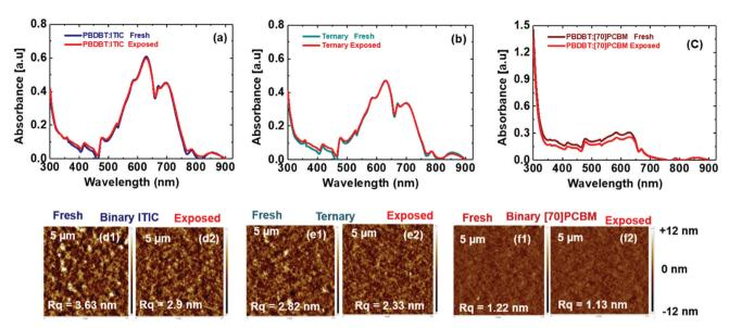
Fig. 3 Absorption spectra of fresh and exposed (2 h) films: PBDB-T:ITIC (a), ternary (b), and PBDB-T:[70]PCBM (c). AFM images of fresh and exposed (2 h) films: PBDB-T:ITIC (d1 and d2), ternary (e1 and e2), and PBDB-T:[70]PCBM (f1 and f2).
