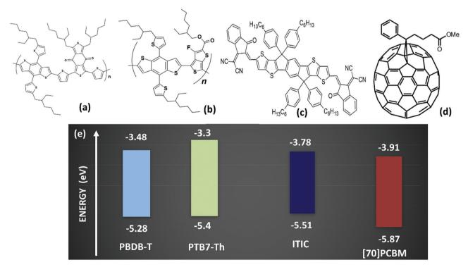
Fig. 1 Semiconductor materials employed: PBDB-T (a), PTB7-Th (b), ITIC (c), [70]PCBM (d) with their corresponding HOMO-LUMO energy levels (e).
