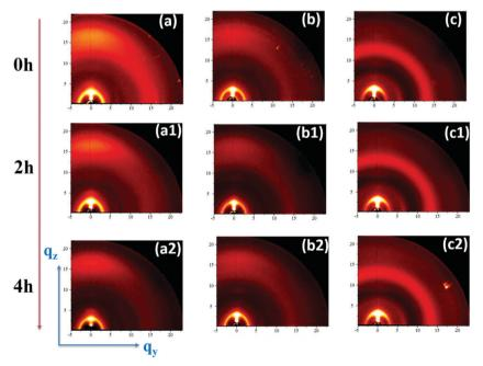
Fig. 4 GIWAXS images of fresh (0 h) and exposed (2 h and 4 h) films: PBDB-T:ITIC (a, a1, and a2), ternary (b, b1, and b2), and PBDB-T:[70]PCBM (c, c1, and c2). Fresh 0 h (a-c), exposed 2 h (a1, b1, and c1) and exposed 4 h (a2, b2, and c2). Note that the intensity scale is the same for all the patterns.
