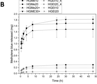
Fig. 8 (A) Released masses of MB after 48 h and (B) release profiles during the first 48 h. There was always a significant difference between the hydrogel types (p < 0.05) unless otherwise indicated by n.s. (not significant).
