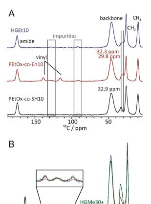
Fig. 6 (A)  $^{1}\text{H}-^{13}\text{C}$  CP/MAS solid-state NMR spectra of the cross-linked hydrogel HGEt10 (blue) as well as the two precursor polymers with thiol and vinyl units and (B)  $^{13}\text{C}$  CP/MAS solid-state NMR spectra of HGMe10+, HGMe20+ and HGMe30+. All experiments were recorded at 14.1 T and 12.5 kHz MAS. For the CP/MAS experiments, a contact time of 2 ms was used.
