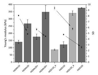
Fig. 7 Young's moduli (columns) and swelling degrees (points) of thiol and cysteine (+) cross-linked hydrogels after 24 h incubation in PBS at 4  $^{\circ}$ C (light grey) or 37  $^{\circ}$ C (dark grey); arrows were added between the same hydrogel types with increasing cross-linking degree to show the correlation between the cross-linking degree and the swelling degree.
