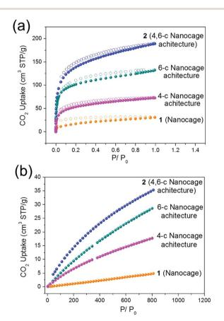
Fig. 4 The  $CO_2$  adsorption isotherms of the nanocage (1), 4-c nanocage architecture, 6-c nanocage architecture and 4,6-c nanocage architecture (2) at (a) 195 K and (b) 298 K.
