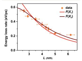
Fig. 4 Measured hot carrier energy loss rates (orange circles) and calculated wavefunction surface fraction (F) of  $X_1$  (red solid line) and  $X_2$  (wine solid line) for  $CsPbBr_3$  NCs of varying sizes.  $F(X_1)$  and  $F(X_2)$  have been appropriately scaled by constant factors.
