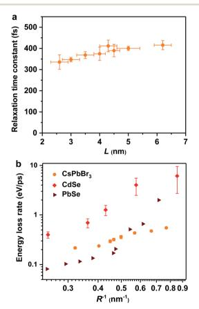
Fig. 2 Hot exciton relaxation time constants (a) and hot carrier energy loss rates (b) of CsPbBr<sub>3</sub> NCs as functions of NC size (orange circles). Note that in order to compare cube-like CsPbBr<sub>3</sub> NCs with previously reported spherical QDs in (b), we define R = L/2 for these NCs. The results for CdSe QDs (red diamonds) and PbSe QDs (wine triangles) are adapted from ref. 23 and 30, respectively.
