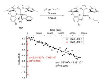
Fig. 3 The plot of  $\ln([Ru]/[Ru]_0)$  vs. time to measure the initiation rates of Ru1-2<sup>46</sup> at -20 °C by monitoring the disappearance of the benzy-lidene signal using <sup>1</sup>H NMR.
