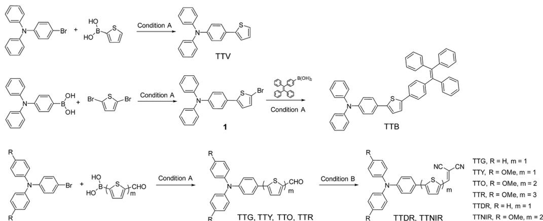
Scheme 1 Synthetic routes to AIEgens with tunable emission colors. Condition A: Pd(PPh<sub>3</sub>)<sub>4</sub>, K<sub>2</sub>CO<sub>3</sub>, THF, H<sub>2</sub>O, 75 °C, 12 h. Condition B: EtOH, malononitrile, 78 °C, 72 h.
