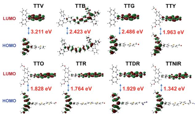
**Fig. 4** Molecular orbital amplitude plots of HOMO and LUMO energy levels of TTV, TTb, TTg, TTY, TTo, TTr, TTDR and TTNIR calculated at the B3LYP/6-31+G(d) level based on the geometries optimized at the TD-B3LYP/6-31+G(d) level.
