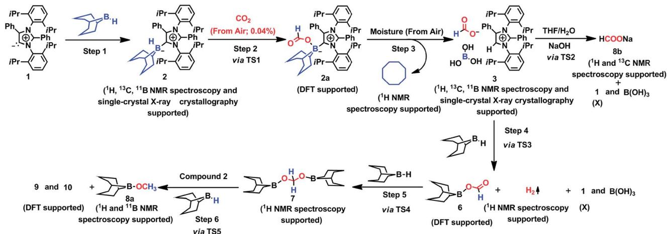
Fig. 6 Mechanistic scheme for the reduction of CO<sub>2</sub> to methoxyborane and sodium formate with 2 in air. For drawings of 9 and 10 see Fig. S3.†
