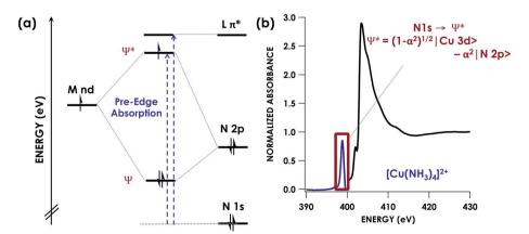
Fig. 1 (a) Simplified energy level diagram showing representative orbitals involved during pre-edge excitations in N K-edge XAS. (b) Representative N K-edge XAS spectrum of  $[Cu(NH_3)_4]SO_4$  with computationally validated pre-edge band assignment.
