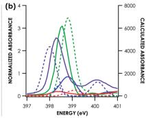
Fig. 2 Example comparison of experimental (solid lines) and TDDFT calculated (a) and DFT/ROCIS calculated (b) (dotted lines) nitrogen K-edge XAS pre-edge features. Calculated spectra are shifted according to individualized fits seen in Fig. 3. Purple =  $\binom{n}{Bu_4N}[RuNCl_4]$ . Green =  $[Mn(bpy)_3](PF_6)_2$ . Blue =  $[Cu(NH_3)_4](SO_4)$ . Red =  $[Zn(en)_3]Cl_2$ .
