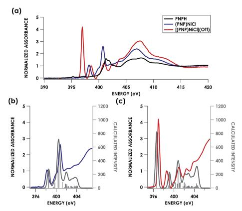
Fig. 7 (a) Experimental N K-edge XAS of PNPH, (PNP)NiCl, and [(PNP)NiCl](OTf). Overlay of experimental (b) (PNP)NiCl (blue) and (c) [(PNP)NiCl](OTf) (red) with TDDFT calculated (grey) N K-edge XAS spectra with energies shifted according to individualized correlation plots seen in Fig. S26† with underlying orbital transitions plotted as sticks in grey.
