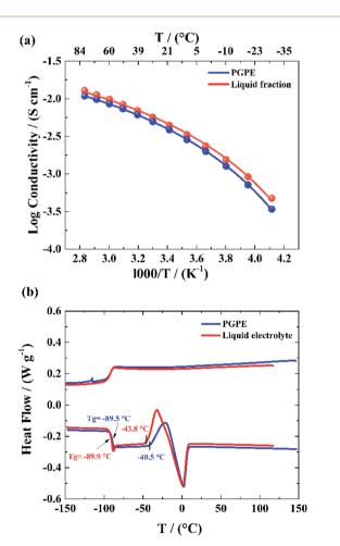
Fig. 2 (a) Ionic conductivity of PGPE and liquid electrolyte. The data points are fitted by VTF function. (b) DSC thermogram, lower curves: first heating ramp and upper curves: cooling trace, both of 10 K min<sup>-1</sup> for PGPE (blue) and liquid electrolyte (red).
