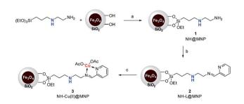
Scheme 1 Synthesis of MNP-supported bifunctional catalyst NH–Cu( $_{\rm II}$ )@MNP (3). Reaction conditions: (a) toluene, N<sub>2</sub>, reflux, 24 h; (b) pyridine-2-carbaldehyde, EtOH, N<sub>2</sub>, reflux, 4 h; (c) Cu(OAc)<sub>2</sub>·H<sub>2</sub>O, acetone, N<sub>2</sub>, RT, 24 h.
