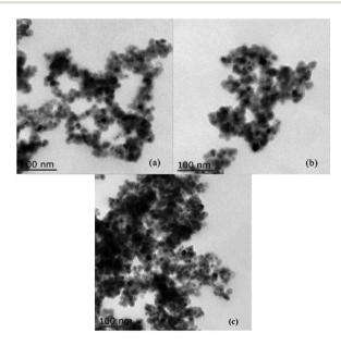
Fig. 5 TEM images of (a)  $Fe_3O_4@SiO_2$ , (b) NH-Cu(II)@MNP and (c) catalyst after being reused six times.
