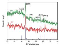
Fig. 4 XRD patterns of (a) Fe<sub>3</sub>O<sub>4</sub>@SiO<sub>2</sub> and (b) NH-Cu(II)@MNP catalyst 3
