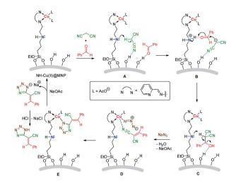
Scheme 2 Plausible reaction mechanism.
