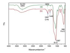
Fig. 3 FT-IR spectra of (a) Fe<sub>3</sub>O<sub>4</sub>@SiO<sub>2</sub> and (b) NH-Cu(II)@MNP.
