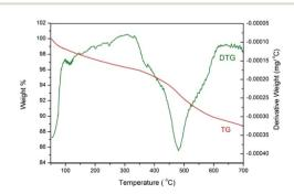
Fig. 7 Thermogravimetric (TG) and derivative thermogravimetric (DTG) curves for NH-Cu(11)@MNP.
