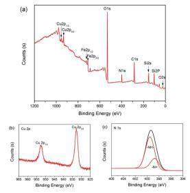
Fig. 6 The XPS spectra of the NH-Cu(II)@MNP catalyst 3. (a) Survey scan; (b) Cu 2p and (c) N 1s.
