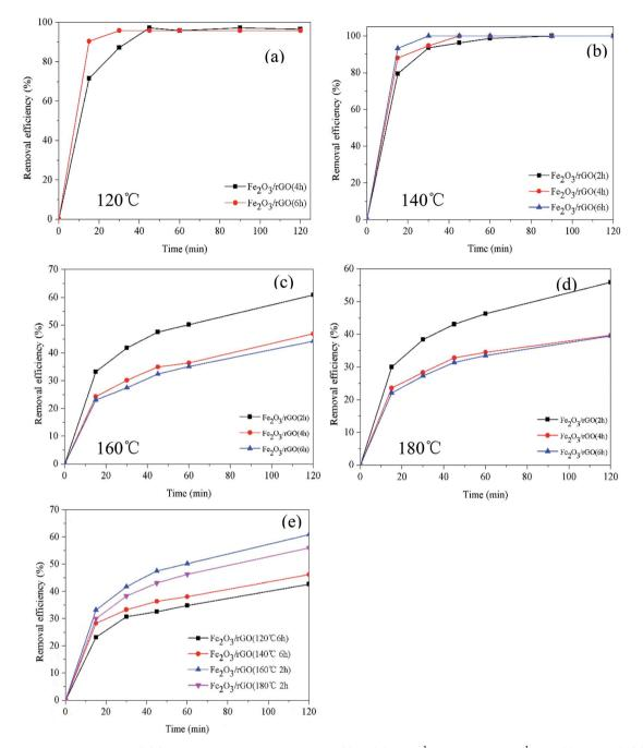
Fig. 1 Effect of preparation time on Cr(vi) removal at different temperatures ( $C_0 = 2.0 \text{ mg L}^{-1}$ ; dosage  $= 0.5 \text{ g L}^{-1}$ ; V = 100 mL; t = 2 h) (a) and (b);  $(C_0 = 5.0 \text{ mg L}^{-1}; \text{dosage} = 0.2 \text{ g L}^{-1}; V = 100 \text{ mL}; t = 2 \text{ h}) \text{ (c) and (d); comparison of the best samples in each group (e) } (C_0 = 5.0 \text{ mg L}^{-1}; \text{dosage})$ = 0.2 g L<sup>-1</sup>; V = 100 mL; t = 2 h).
