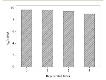
Fig. 10 Regeneration test of the Fe<sub>2</sub>O<sub>3</sub>/rGO (dosage = 0.2 g L<sup>-1</sup>;  $C_0$  = 5.0 mg L<sup>-1</sup>; V = 50 mL;  $t_{\rm removal}$  = 3 h; 0.1 mol L<sup>-1</sup> NaOH, desorption agent;  $t_{\rm desorption}$  = 3 h).
