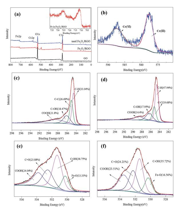
Fig. 6 The spectra survey scans of GO, Fe<sub>2</sub>O<sub>3</sub>/rGO and used Fe<sub>2</sub>O<sub>3</sub>/rGO (a); Cr 2p spectra of used Fe<sub>2</sub>O<sub>3</sub>/rGO (b); C 1s spectra of unused Fe<sub>2</sub>O<sub>3</sub>/rGO (c); C 1s spectra of used Fe<sub>2</sub>O<sub>3</sub>/rGO (d); O 1s spectra of unused Fe<sub>2</sub>O<sub>3</sub>/rGO (f).
