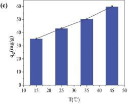
Fig. 9 Effect of pH on Cr(vi) removal ( $C_0 = 16.63 \text{ mg L}^{-1}$ ; dose of Fe<sub>2</sub>O<sub>3</sub>/rGO = 0.4 g L<sup>-1</sup>;  $T = 25 \pm 1 \,^{\circ}$ C; t = 36 h; 140 rpm) (a); effect of the initial Cr(vi) concentration (b); effect of the temperatures (c) (dose of Fe<sub>2</sub>O<sub>3</sub>/rGO = 0.4 g L<sup>-1</sup>; pH = 2.2; t = 36 h; 140 rpm).
