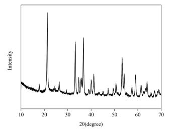
Fig. 4 The XRD pattern of Fe<sub>2</sub>O<sub>3</sub>/rGO.
