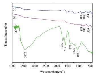
FTIR spectrum of GO (a), Fe<sub>2</sub>O<sub>3</sub>/rGO (b) and used Fe<sub>2</sub>O<sub>3</sub>/rGO
